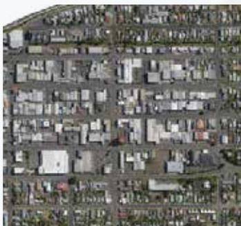
Routine operations comfortably capture high resolution coverage of 4-6 square km per flight. Task areas anywhere from 12-30 km<sup>2</sup> are routinely viable within one operating day.
